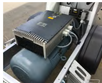
The 22 kW Electric motor
