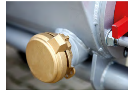
Large opening for cleaning
