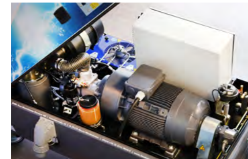
The 30 kW variable frequency electric motor
